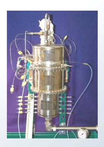
25 kW<sub>th</sub> ATR w. fuel/air/steam injector, igniter, steam generating HX, sulfur trap, WGSR
