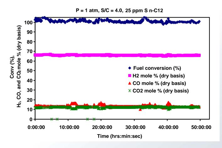
W. 25 ppm<sub>w</sub> S n-C12 (DBT-doped), conversion was stable at 100% & H<sub>2</sub> conc. was steady.
