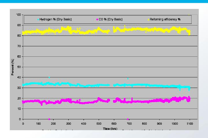
JP-8 w. low S (Average ~15  $ppm_w$  S) Operated with I  $kW_e$  SOFC stack – Stable Operation w/o coking for I 100 hours
