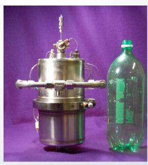
5 – 10 kW<sub>th</sub> reformer integrated w. fuel/air/steam injector, igniter, steam generating HX, sulfur trap
