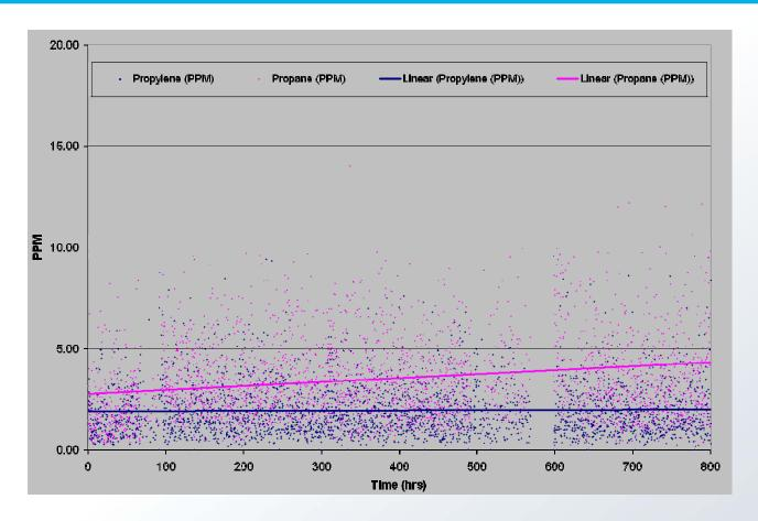
Propylene and propane <10 ppm<sub>v</sub> for up to 1100 hrs; Ethylene and ethane were not detected by GC (<5 ppm<sub>v</sub>)
